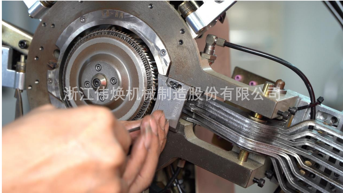
装上平板放梭板 put on the plain yarn feeder plate
