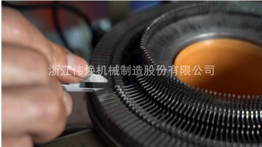
另外一半装入低脚生克片 left space for plain sinker S
