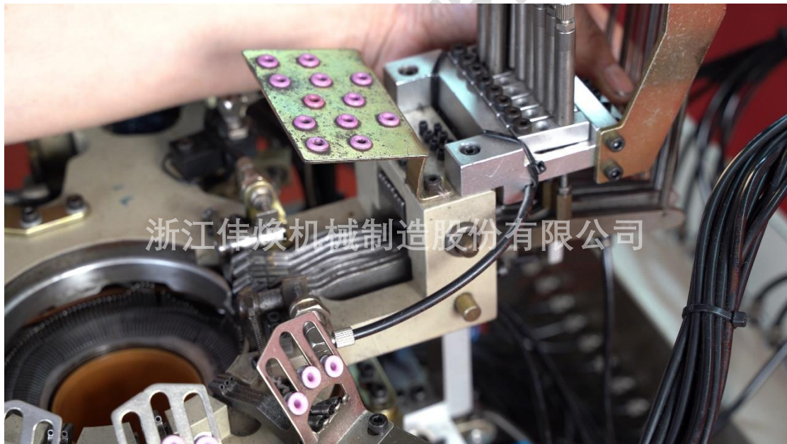
调整梭子高低前后 adjust the feeders position
